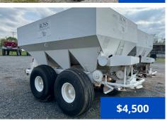
AGCO Willmar S800, 50 ft dual spinner spreader with standard equipment, 409 SS spreader box with 8-ton capacity, hydraulic rope control, 77 in track width with 4-wheel brakes, (4) 19L-16.1SL tires.
