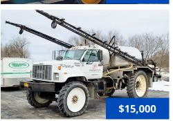
**1996 Stahly GMC TopKick**, 8205 hours, 73,454 miles, GMC chassis, CAT 3116 diesel engine, automatic trans., 1450 gal. SS tank, 60 ft booms with poly boom lines, 15 in. nozzle spacing, 5-section shutoff valve, single body nozzles, Raven SCS 460 controller, SS chemical eductor, AM/FM, A/C, air ride seat, fenders, 320/85R34 Michelin Agribib tires.
