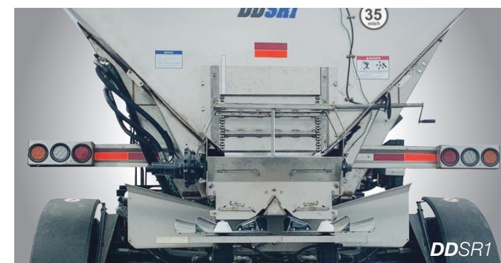
SR1: Reverse Rotation, Single chain (1-Section)
