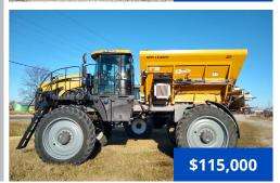
**2015 AGCO Rogator RG1300B,** 2800 hours, AGCO diesel turbo engine, 4-speed hydrostatic auto. trans., AGCO adjustable axles, 4WS, painted 409SS New Leader L4000G4 spreader body, Raven Viper Pro, AutoSteer, A/C, AM/FM radio, air ride seat, 380/90R46 tires, front (50% remains) rear (45% remains), includes a set of floater tires. New roller, bearings, and straight belt.
