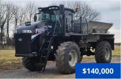
**2015 GVM E325 Prowler,** 3992 hrs., Cummins QSL 8.9L 325 hp diesel engine, 1010 ft-lb torgue, auto. ZF WG 210 6-speed powershift trans, 99 in. axles, variable coil spring suspension, combo ready, painted 409 SS New Leader L4000G4 spreader body, bin level sensor, rear camera, Raven Viper Pro, reverse pitch fan, A/C, AM/FM radio, air ride seat, Firestone 380/90R46 tires.
