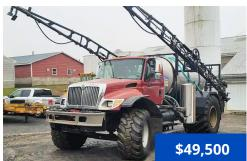
2004 International DT 7400, 3038 hrs., MaxxForce 300 hp diesel engine, Eaton Fuller 10-speed trans., Miller 1200 gal. SS tank, 70 ft booms with SS boom lines, 30 in. nozzle spacing, 7-section shutoff valve, single body nozzles, Ag Leader 1200 controller, SS chemical eductor, foam marker, A/C, AM/FM radio, air ride seat, fenders, includes front 650/55/R26.5 Alliance (75% remains) and rear 105/50/R32 Trelleborg tires (90% remains). Product pump replaced in 2023, great condition!
