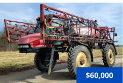
**2007 Case IH Patriot SPX3320,** 4309.4 hrs., Case 240 hp diesel engine, hydrostatic trans., 1000 gal. SS tank, 90 ft. booms with 20 in. nozzle spacing, SS chemical eductor, active suspension, Raven SCS 4400, Cruiser II, A/C, AM/FM radio, air ride seat, fenders, row crop tires.
