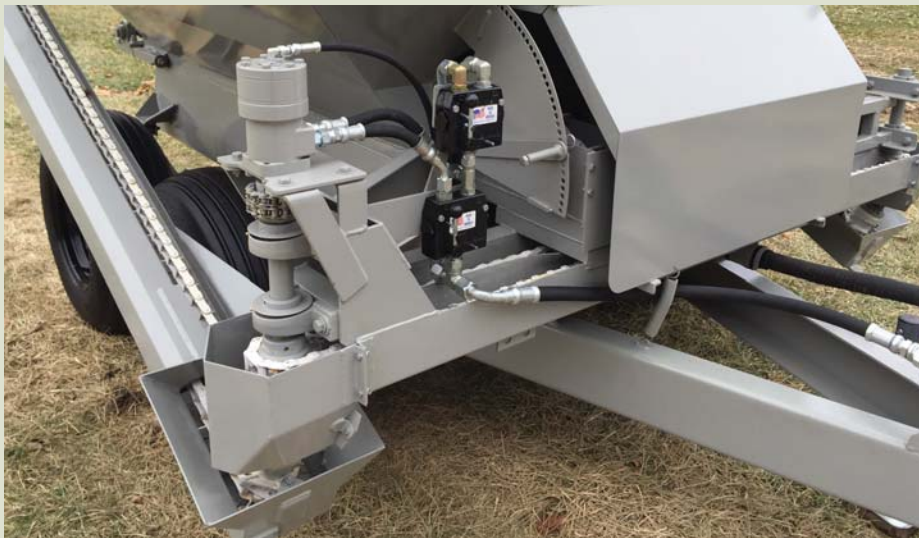
Top mounted drive motors keep material safely away from chemicals
