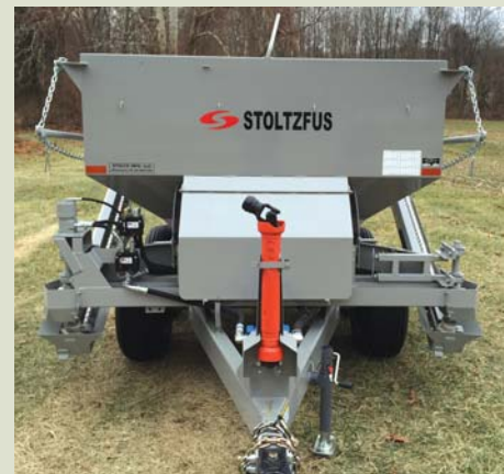
Booms fold easily for transport and storage
