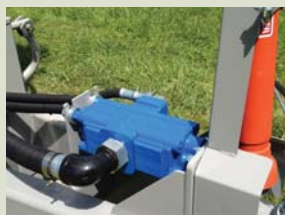
Self-contained PTO hydraulics reduces the strain on your tractor's hydraulic system
