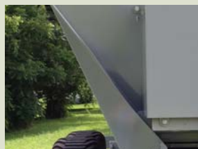
Steep, 53° hopper side slopes for enhanced material flow
