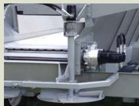
Spinner motors mounted out of the flow of corrosive materials for increased life
