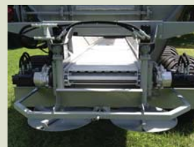
Double gearboxes and hardened conveyor drive shaft double the breakout power for heavy loads of damp, stockpiled lime
