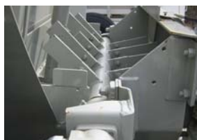
Shredder to chop up clumps and give a smoother flow of material onto the spinners
