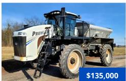
2017 GVM E330AA Prowler, 5214 hrs., Cummins Tier 3 OSL 9L 330 hp turbo diesel engine, Funk DF250 11-speed powershift trans., 93-120 in wheel spacing, Dromos adjustable axles, 409 SS New Leader L4000G4 10-ton spreader, Raven Viper Pro, SmarTraxx, A/C, AM/FM radio, air ride seat, beacon lights, CleanFix fan, Firestone VF380/90R46 tires (40% remains).
