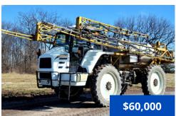
**2011 GVM 9275 Prowler,** 6766.9 hours, Cummins QSB6.7L 275 hp diesel engine, Funk 10-speed powershift trans., 1450 gal. SS tank, 70/90 ft booms with SS boom lines, 15 in. nozzle spacing, 5-section shutoff valve, triple body nozzles, Raven Viper 4+, parallel swatching, 3 sensor AutoBoom, AccuBoom, A/C, AM/FM radio, air ride seat, 380/90R46 Trelleborg tires (30% remains), includes set of floater tires not pictured.
